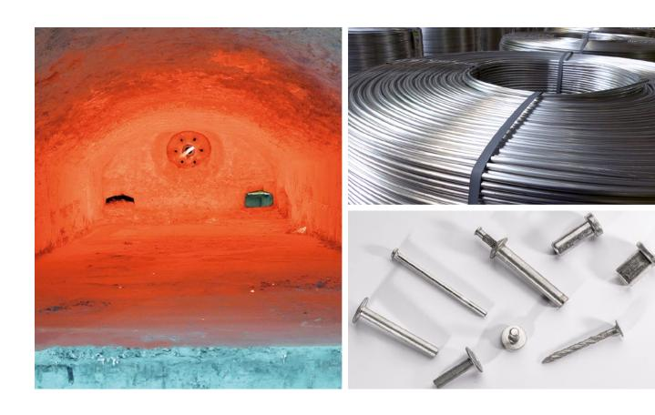
Redraw Rod – Continuously Cast and Rolled
